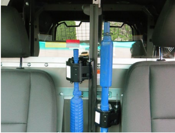
Tri-Lock Vertical Partition Mount Gun Rack in the Ford Police Utility Interceptor
