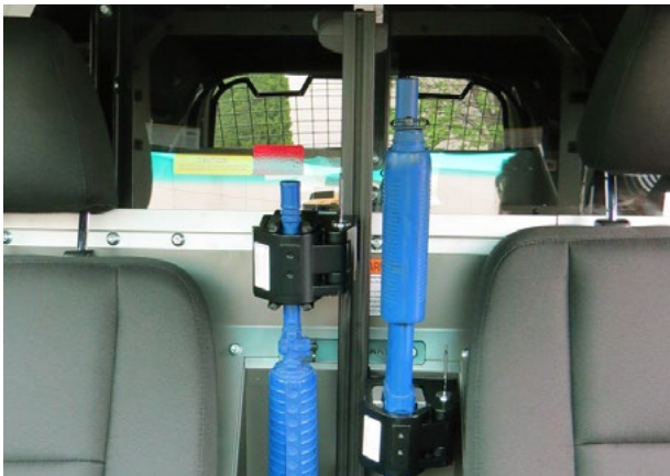
Vertical Partition Mount Gun Rack shown in the Ford Police Utility Interceptor
