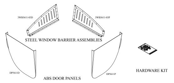
THIS WINDOW BARRIER IS ONLY USED WITH #DP56C11 ABS DOOR PANEL. Use #WB56NPC11P with OEM door panel.
