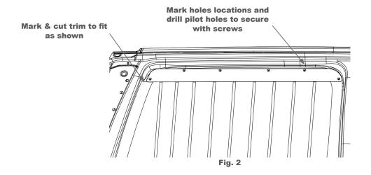
E. Once the window trim is re-installed then the window bars can be install and secured to the vehicle. Re-install the window bars and use the door lock to locate the position.
