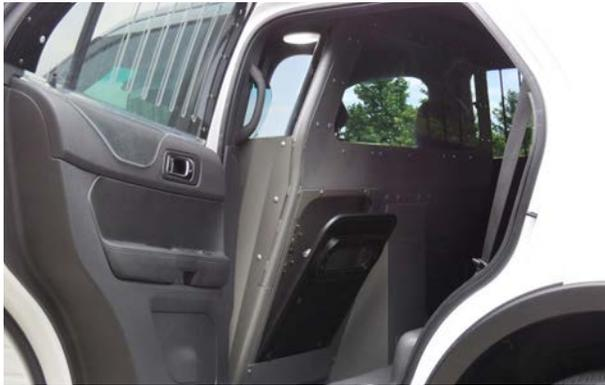
VIPER™ Shield deployed upon releasing T-handle
