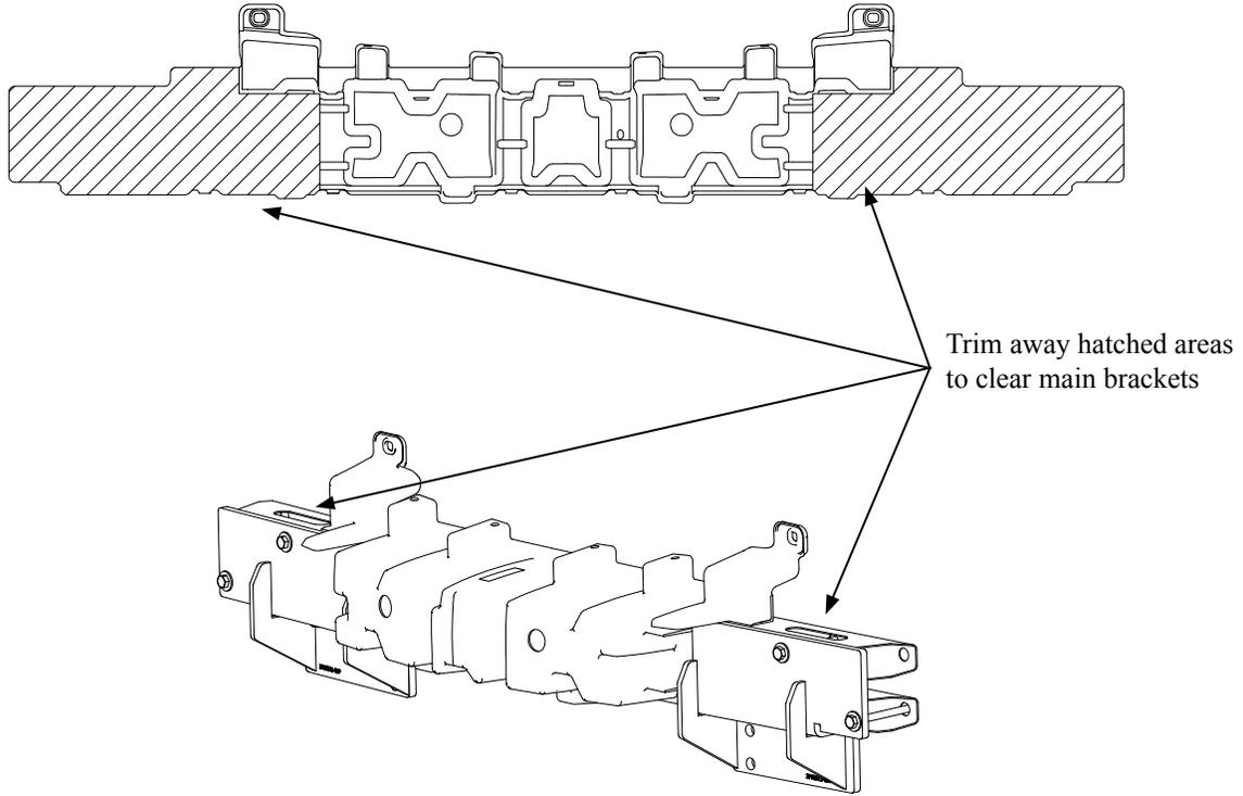
6. Reassemble the plastic crush bumper to the metal bumper. Replace the fascia to the front of the vehicle and mark where the lower brackets interfere with the lower grill opening. Cut the grill to clear the brackets. See Fig. 4.
