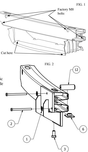
pro-gard.com 800.480.6680 5. Retrieve the vehicle's plastic crush bumper and trim to fit per Fig. 3.
