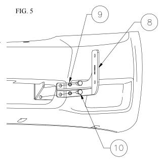
Install the lower bracket (8) on driver side of car, using 1/2-13 x 1-1/2" bolt (10), and 1/2" split ring washer (9). See Fig. 5 Repeat for passenger side using bracket (5).
