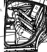
pro-gard.com 800.480.6680 A. Remove the T15 Torx screw from the rear tab of the Rear Door Scuff Plates and then remove the Rear Door Scuff Plates on the Driver and Passenger-side. These will be reinstalled after the ABS Floor Pan Installation. (See Fig. 3)
