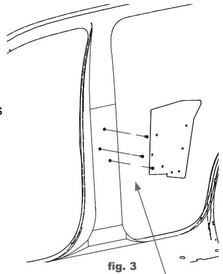
Set recess panel in vehicle before partition installation
