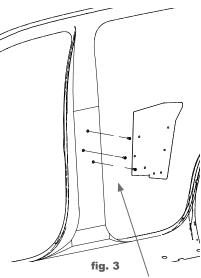
Place 3X36 bolt into hole at this time. Access will be restricted later.
