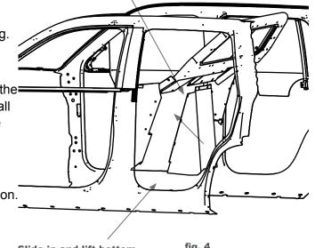
Slide in and lift bottom towards front of vehicle fig. 4
