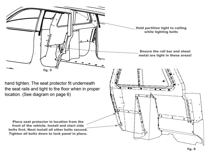
D. Place the passenger's side bucket seat protector (3SP57SST15 - P) in the vehicle from the front and set in location. Get all bolts started and tighten to secure. (See main diagram on page 5)
