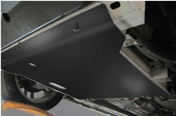
Skid Plate installed on a Chevy Caprice
