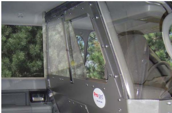
Passenger 1/2 sliding polycarbonate window shown in the Ford F150
