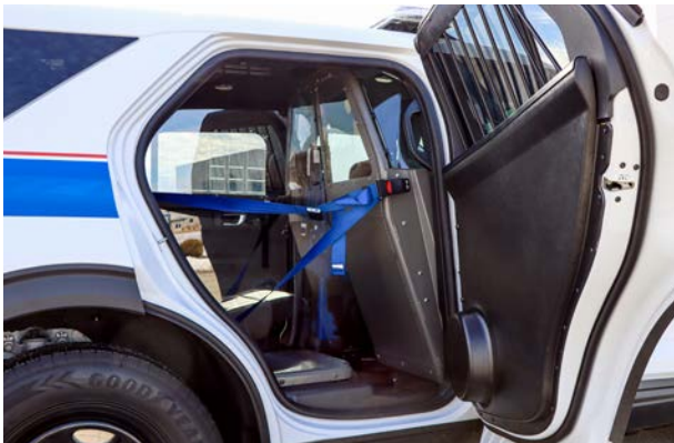
P1300, shown with passenger side custom molded replacement door panel
