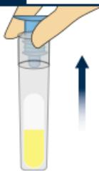
Ensure that the test tube remains upright in order to avoid the ampule falling out of the tube.
