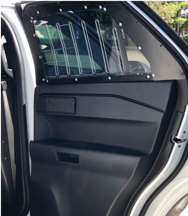
Door Panel Cover Plates eliminate rear access to the door handle and window controls on the 2020 - current Ford Interceptor Utility
