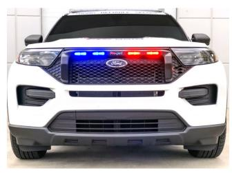
The lightweight Command Grille® easily mounts onto the existing grille of the 2020 Ford Police Utility Interceptor.
