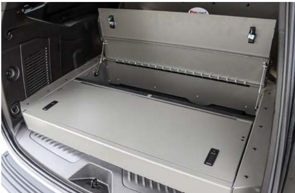
Second compartment is designed to hold equipment/gear and has a non-locking lid.
