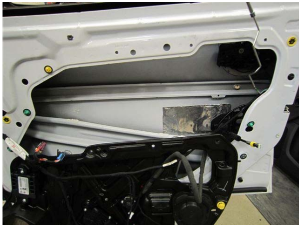
Figure 7: Remove door insert.
