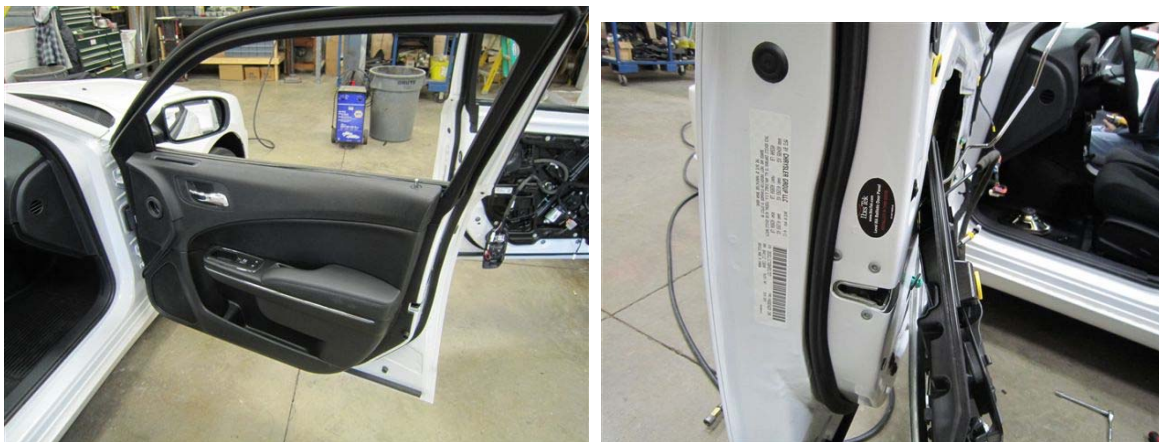
Figure 22, 23: Reinstall door trim and apply door trim decal as shown.
