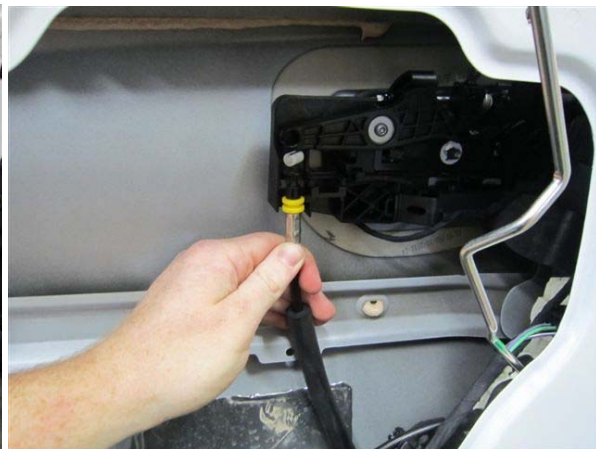
Figure 8: Disconnect outside door latch cable.
