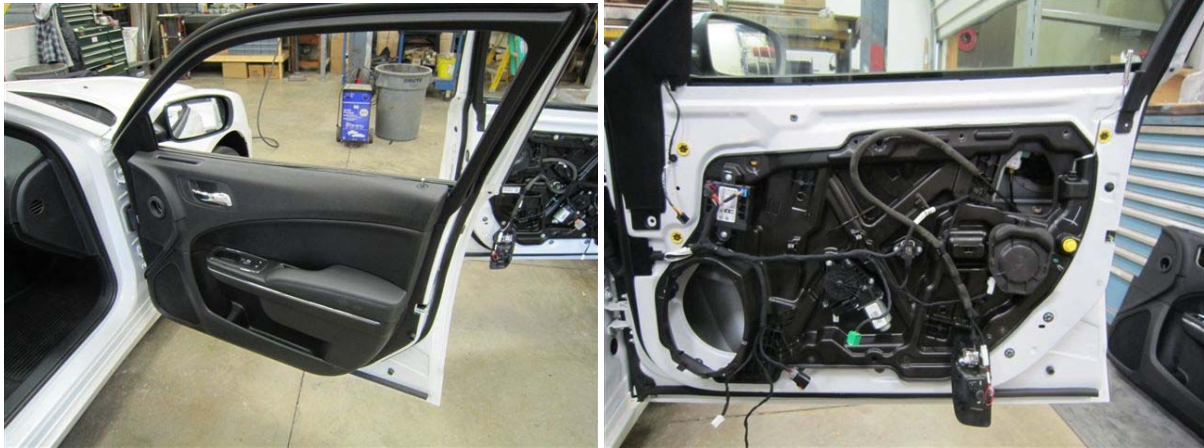
Figure 3, 4: Remove door trim. Disconnect speaker
