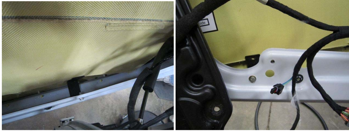
Figure 18, 19: Assemble lower bracket through use of existing hole in door as shown.
