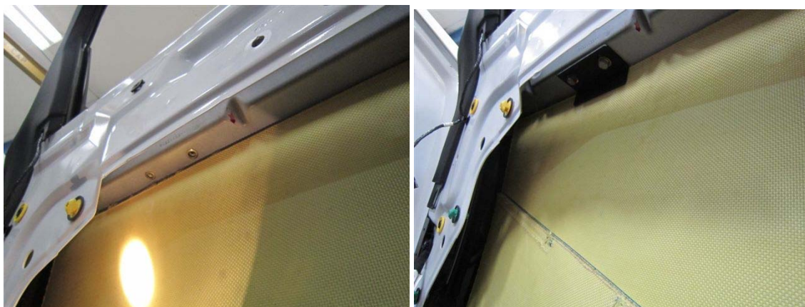
Figure 16, 17: Install riv nuts and assemble Upper Bracket to door.
