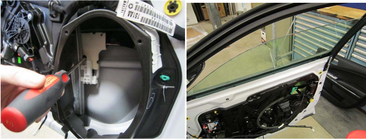
Figure 5,6: Push in tab to remove window from track. Remove glass from door.
