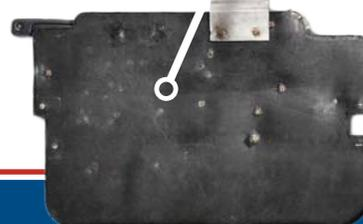
Actual test results on a standard Ford Crown Victoria door with a Pro-gard Level IIIA NIJ, Ballistic Panel
