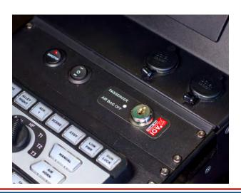
Our patented Front Passenger Airbags On/Off Control Switches provide officers the solution to perform without the threat of damage to themselves and vehicles when their airbag is deployed. The installation and use of the front passenger switch eliminates the dangerous conflicts between aftermarket equipment mounted on the dash that may interfere in the airbag deployment zone.
