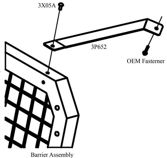
E. Attach the lower mounting brackets to the Barrier using the Phillips head bolts (3X05A) and whiz nuts (3X16) through the existing holes in the Barrier. See Fig. 2
