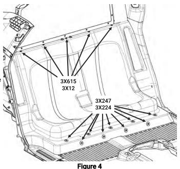
E. Reinstall the OEM lower seatbelt fasteners that were removed in section IV step D. Use a T50 torx to torque to factory specifications. If using the OSB system, this fastener helps to cover a hole in the trim.
