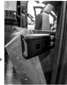
E. Locate (1) Partition Buckle [30SB000001], (2) 1/4" carriage bolts [3X36], (2) 1/4" whiz nuts [3X16Z], and (2) plastic nut caps [3X145]. Position the Partition Buckle in the desired belt park position on the passenger Partition Mounting Plate, mark the location for (2) holes, drill the holes, then attach the buckle to the partition with the hardware gathered. Repeat for the driver side if using a full OSB system. Figure 6 shows the recommended position for the Partition Buckles.
