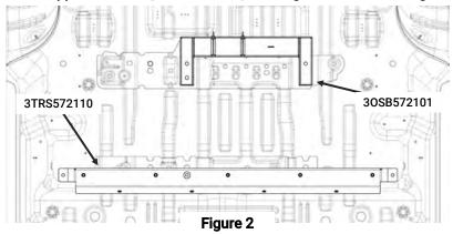
Ensure the Center Support Bracket is sitting flat on the sheet metal floor pan of the vehicle and then install (3) of the OEM bolts that were removed from the seats.
