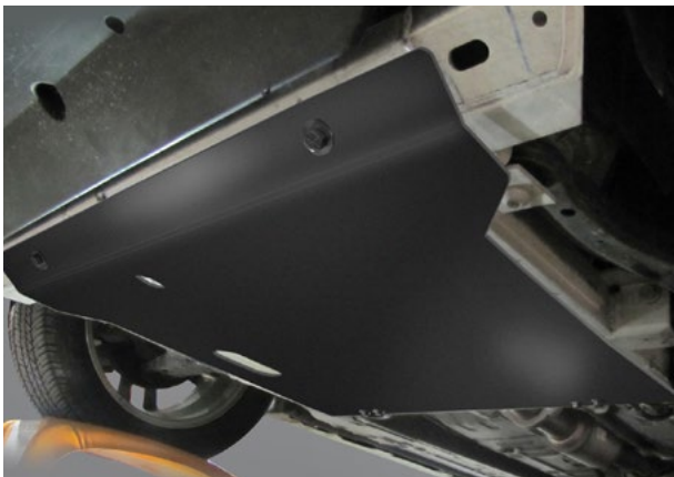
Skid Plate installed on a Chevy Caprice
